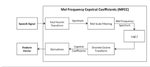
Fig. 2. Diagram demonstrating the steps for calculating MFCCs (Lutter 2014).
