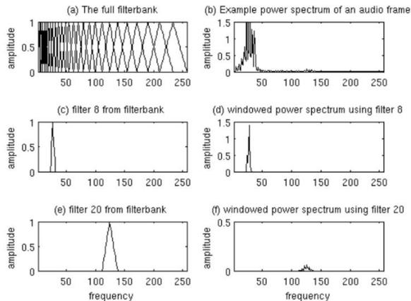
Fig. 1. Diagram demonstrating the Mel-Scale filtering process (Lyons 2012).
