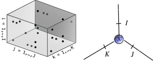
Fig. 2. (a) A third-order sparse tensor; (b) Tensor network diagram for a third-order tensor.
