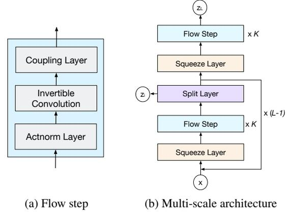
Figure 2. Overview of architecture of generative flows. We can design the flow step by selecting a suitable convolutional layer and a coupling layer based on the task. Glow (Kingma & Dhariwal, 2018) uses  $1 \times 1$  convolutions and affine coupling.
