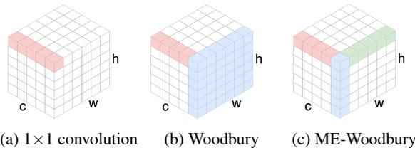
Figure 1. Comparison of three transformations. The  $1 \times 1$  convolution only operates along the channel axis. The Woodbury transformation operates along both the channel and spatial axes, modeling the dependencies of one channel directly via one transformation. The ME-Woodbury transformation operates along three axes. It uses two transformations to model spatial dependencies.
